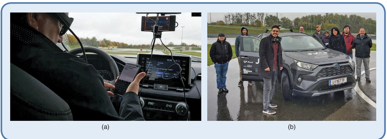
FIG 2 Field tests with an JKU-ITS automated vehicle at the Driving Technology Center at Österreichische Automobil-, Motorrad- und Touring Club, Marchtrenk, Austria. (a) A driver performing a non-driving-related task (NDRT) during a real-world evaluation of the impact of automated driving system technology on driver gaze behavior, reaction time, and trust. (Source: Cristina Olaverri-Monreal; used with permission.) (b) The team at JKU-ITS during the field test. (Source: Stefan Neubauer; used with permission.)
