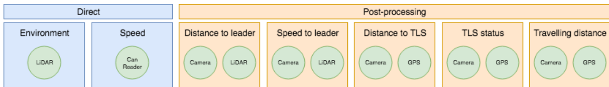
Figure 3 – Data schematics for the instrumented vehicle and the data post-processing pipeline.
